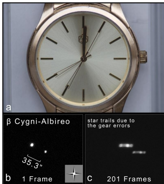
Figure 3. The gear errors affect the pointers' position of a clock and the stars' position on the telescope's field (telescope adapted on an equatorial mount). a – the pointer of the seconds aims at the dial subdivision (subdivision 1). In the opposite position, the pointer of the seconds should aim on the subdivision '7' for the 35 th sec and on '8' for the 40 th sec. Because of the pointer's (or
