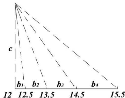
**Figure 11.** Scheme illustrating the location of the segments  $b_i$  formed by the intersection of adjacent hour lines from 12 to 15,5 o'clock with a line perpendicular to the noon line,  $c$  - the distance from the place of attachment of the gnomon to the line perpendicular to the noon line.
