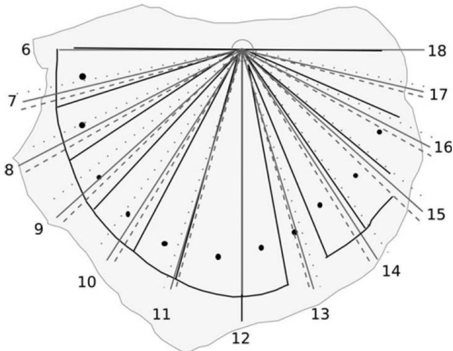
**Figure 3.** Limestone tile from the Valley of the Kings, drawing with applied hour lines calculated for a vertical sundial with a horizontal gnomon. The noon line was chosen as the zero point. The lines on the limestone tile are shown in the drawing as black solid lines, the hour lines calculated for the equinox are shown as gray solid lines, for the summer solstice - gray dotted lines, for the winter solstice - gray lines of dots [11].
