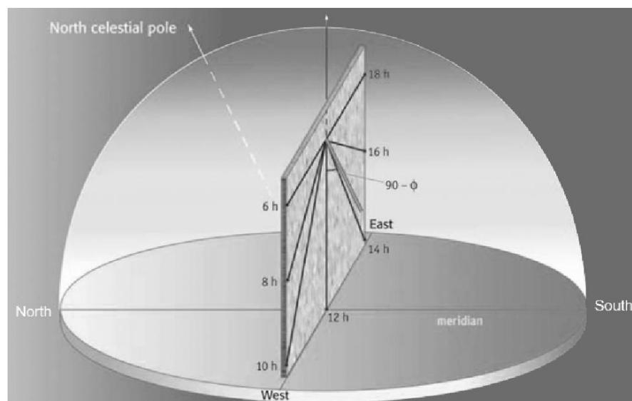
**Figure 4.** Scheme illustrating the principle of operation of a vertical sundial with an inclined gnomon [14].
