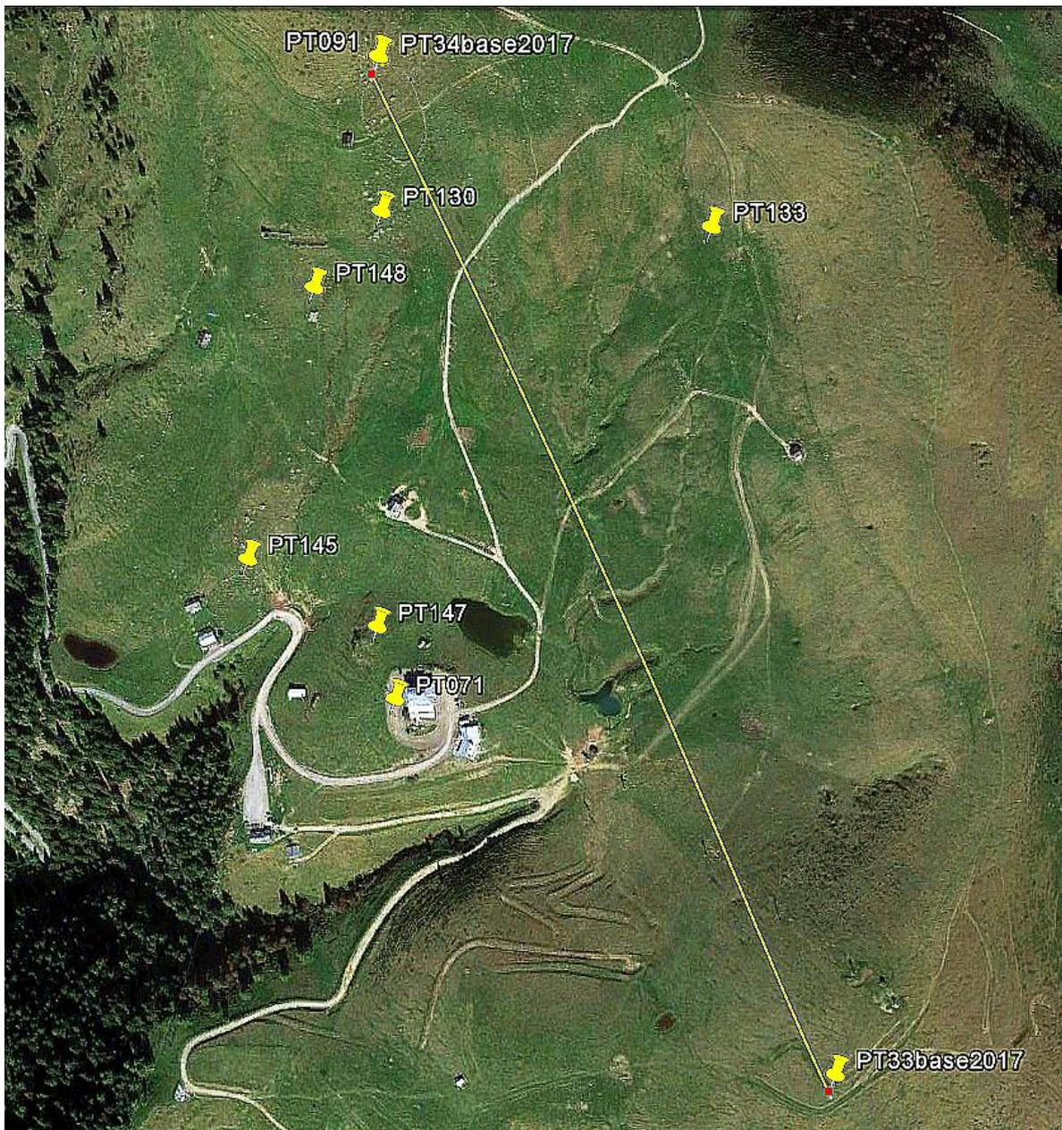
**Figure 3.** The GPS baseline materialized at the Piani del Monte Avaro and used to calibrate the magnetic azimuths measured by transforming them into astronomical azimuths (photo from Google Earth).
