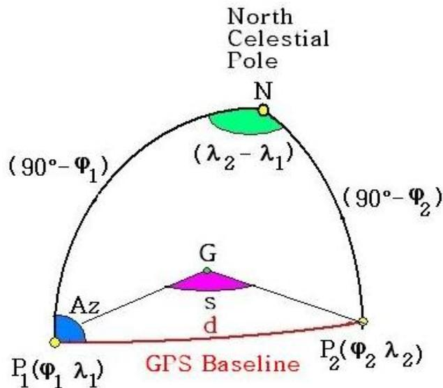
**Figure 4.** The spherical triangle solved in order to carry out the geodetic/astronomical azimuth of orientation of the baseline P1→P2.
